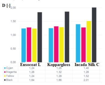
Fig. 2. Diagrams of optical densities of printed images
