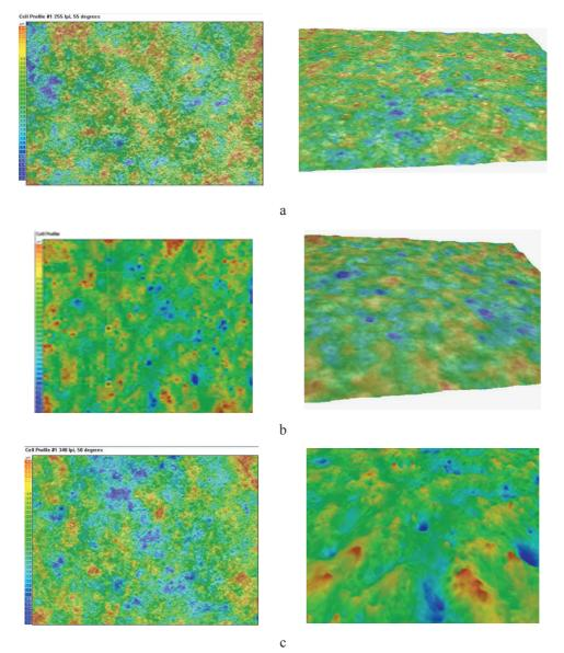
Fig. 3. Topography of the surface structure of imprints and their 3D models on cardboard: Koppargloss (a); Incada Silk C (b); Ensocoat L(c)
