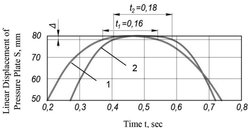
Fig. 5. Graphs of the dependence of the movement of the pressure plate on time in the cardboard die-cutting zone in the wedging mechanisms: the existing (1), the proposed double-crank (2)
