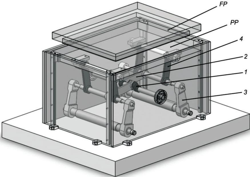
Fig. 2. 3D model of the existing wedging mechanism of the pressure plate drive
