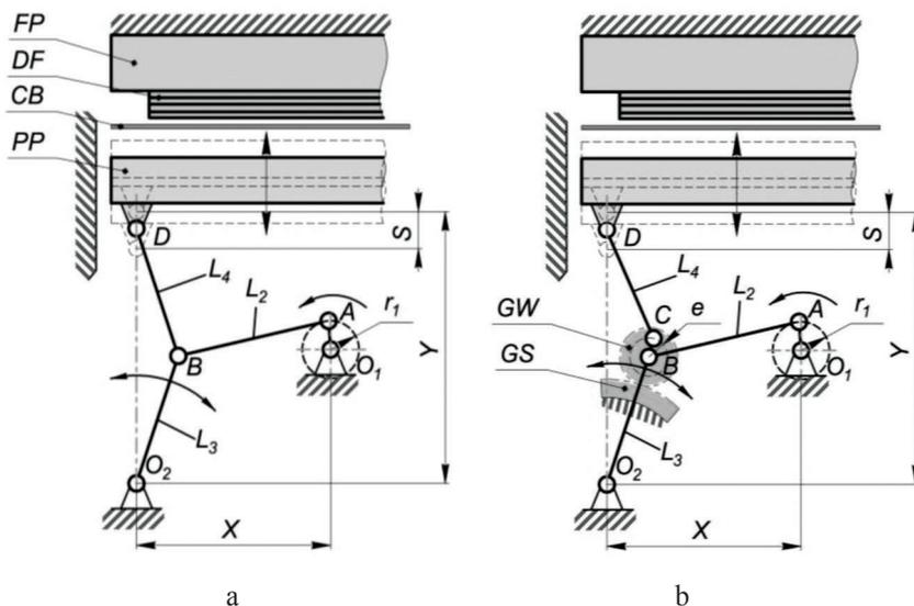
Fig. 1. Calculation schemes of the left circuit for the synthesis of geometric parameters: a) existing wedging mechanism; b) double-crank wedging mechanism with the additional driven crank
