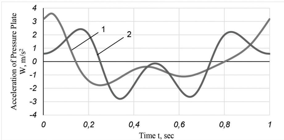
Fig. 7. Graphs of the dependence of the acceleration of the pressure plate on time in the wedging mechanisms: existing (1), proposed double-crank (2)
