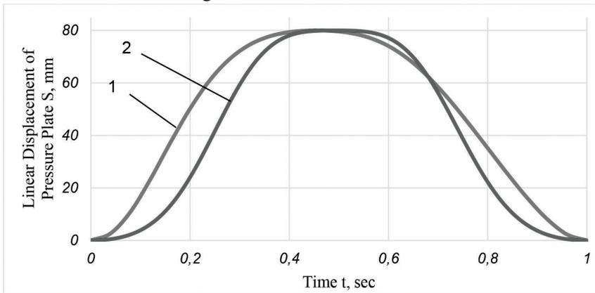
Fig. 4. Graphs of the dependence of the displacement of the pressure plate on time in the wedging mechanisms: the existing (1), the proposed double-crank mechanism (2)
