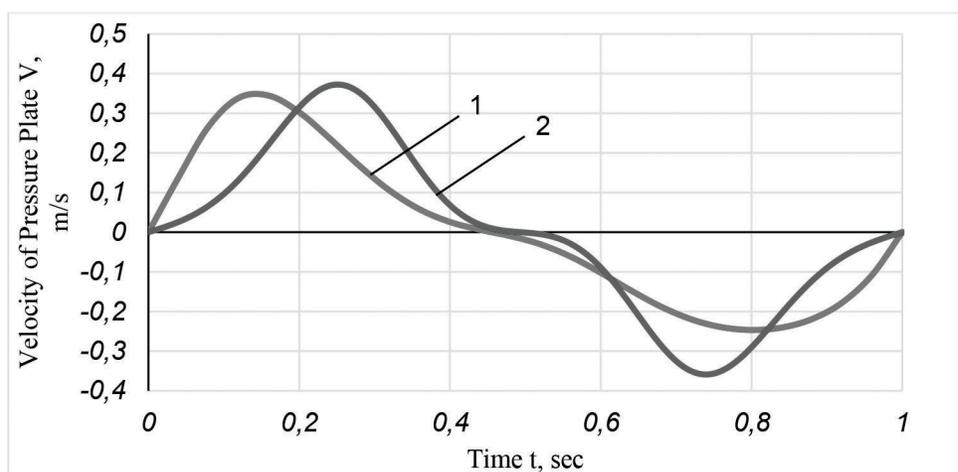
Fig. 6. Graphs of the dependencies of the velocities of the pressure plate on time in the wedging mechanisms: existing (1), proposed double-crank mechanism (2)
