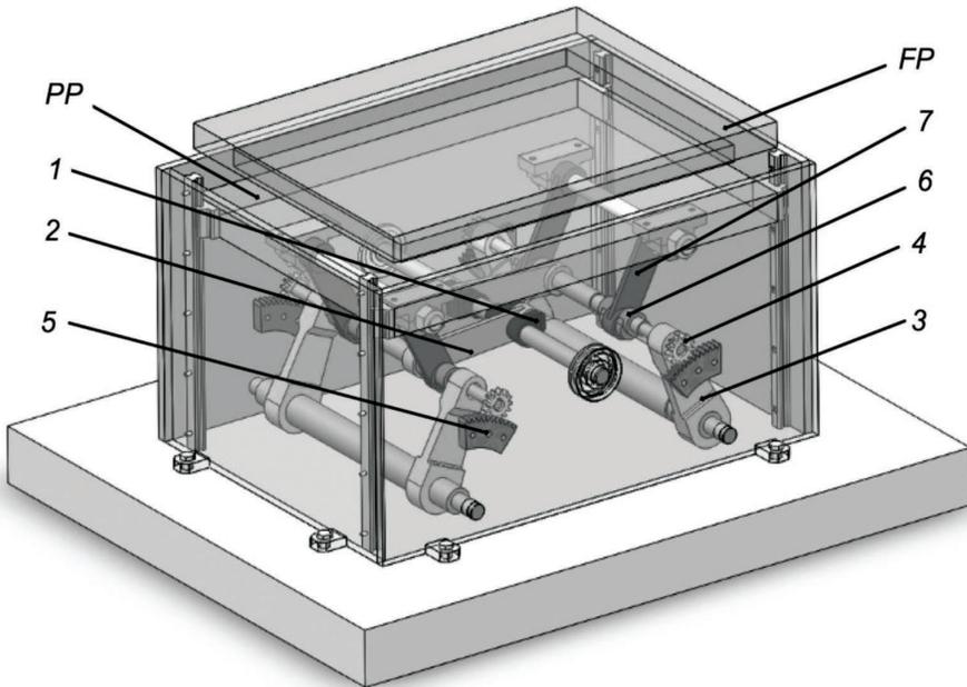
Fig. 3. 3D model of the wedging mechanism with an additional driven crank of the pressure plate drive
