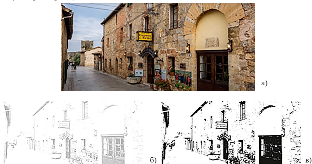
Fig. 4. Application example of the developed TAC control methodology: a) original [7], b) areas exceeding 240% TAC, c) enhanced visualization of over-limit areas for further processing
